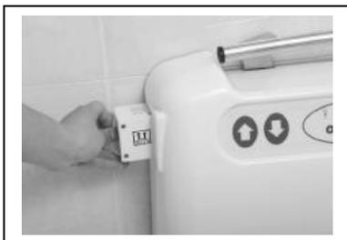
The battery chamber is located at the left upper corner of the belt housing case. Please make sure that the battery is dry and the 'This side up' sign is in a position like shown in the left picture, before you place the battery into the chamber.
